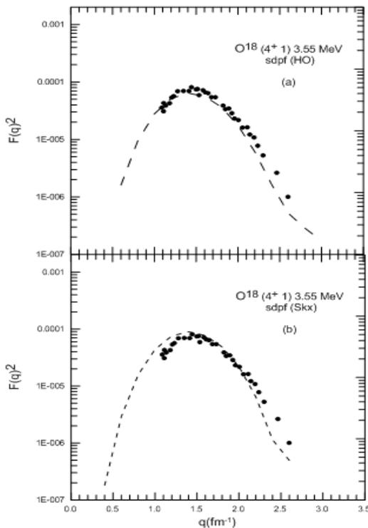
Figure 1. The isovector electron scattering form factors for the  $4^+1$  (3.55 MeV) state in  $^{18}\text{O}$ . The solid curve represent the calculation with sdpf model space. The upper panel represents the form factors that calculated with HO potential for radial part of the single-particle matrix elements, while the lower panel represents those of the Skx interaction. The data are taken from Ref. [20]
